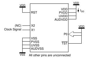
Figure 24-2. I<sub>DL</sub> Test Condition, Idle Mode
