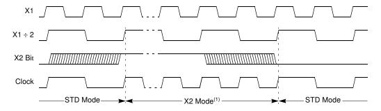
Note: 1. In order to prevent any incorrect operation while operating in X2 mode, user must be aware that all peripherals using clock frequency as time reference (timers, etc.) will have their time reference divided by 2. For example, a free running timer generating an interrupt every 20 ms will then generate an interrupt every 10 ms.
