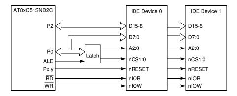
Figure 17-4. IDE Device Connection Example 2
