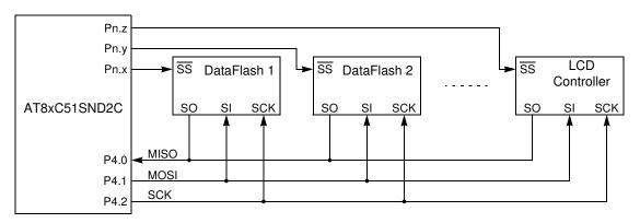
Figure 19-2. Typical Slave SPI Bus Configuration
