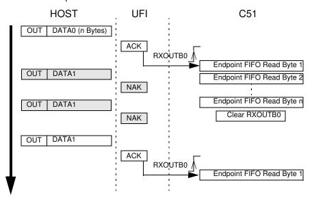
An endpoint should be first enabled and configured before being able to receive Bulk or Interrupt packets.
