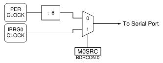
Figure 20-7. Baud Rate Formulas (Mode 0)
