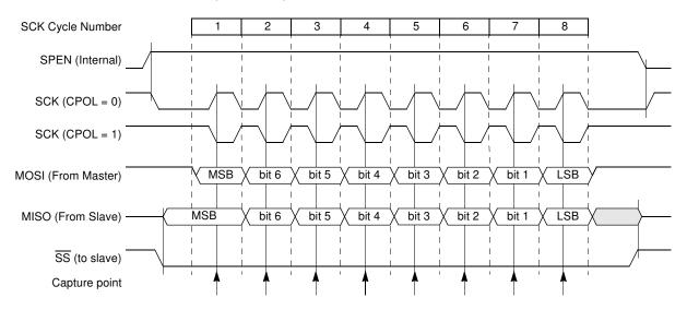
**Figure 19-6.** Data Transmission Format (CPHA = 1)
