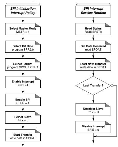
Figure 19-10. Master SPI Interrupt Flows
