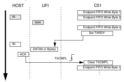
An endpoint should be first enabled and configured before being able to send Bulk or Interrupt packets.
