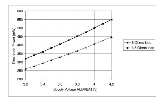
Dissipated Power [mW] ▲ 8 Ohms load ■ 6.5 Ohms load Output Power [mW]
