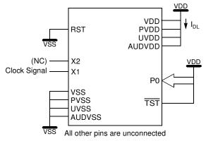
Figure 24-3.  $I_{PD}$  Test Condition, Power-Down Mode
