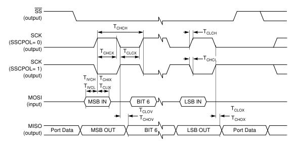
Note: 1. SS handled by software using general purpose port pin.
