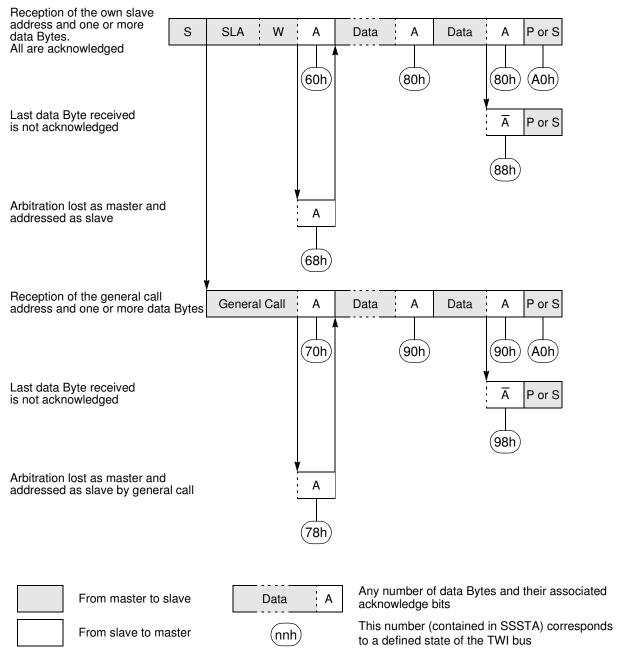
Figure 21-6. Format and States in the Slave Transmitter Mode
