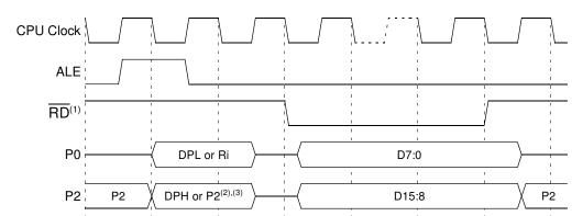
Figure 17-1. IDE Read Waveforms
