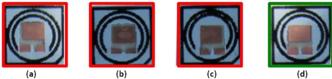
Figure 28. During PCB manufacturing poor positional control of the solder mask layer with respect to the top metallization layer can impact the actual pad dimensions on the PCB. The four pictures in this example were all taken from the same physical 4-up PCB. The anode and cathode dimensions for positions (a) – (c) on this PCB are smaller than originally designed. Only the pad dimensions for position (d) were in specification.
