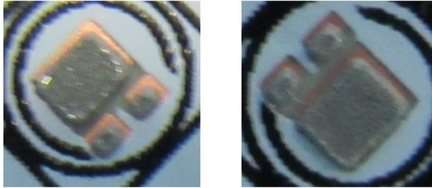
Figure 15. A poorly placed stencil may cause some of the solder paste to be deposited onto the solder mask, reducing the amount of solder paste which is available on the pads to establish a strong solder joint. In this example, the silk screened circles within the LUXEON package outline may also lift the stencil from the solder mask, compromising the quality of the solder paste deposition process.
