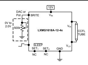
Figure 1 – Brightness Control (output current set to maximum)
