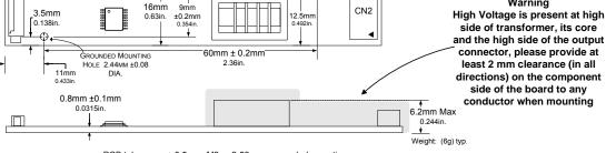
PCB tolerances ± 0.5mm, M2 or 2-56 recommended mounting screws All dimensions are in millimeters, inches are for reference only
